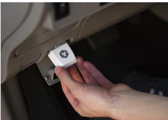
**Figure 4: Bluetooth device in OBD-II port<sup>31</sup>**
