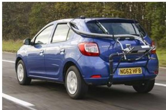
**Figure 2: Real driving emissions testing<sup>16</sup>**
